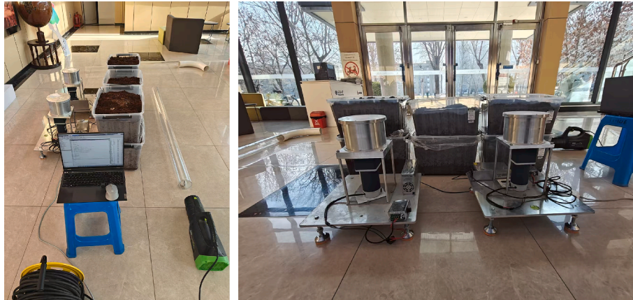
Fig. 14. Pipeline localization experiment photo with soil-shielded environment.
