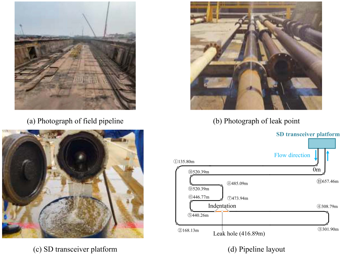
Figure 5. Pipeline leak detection experiment.
