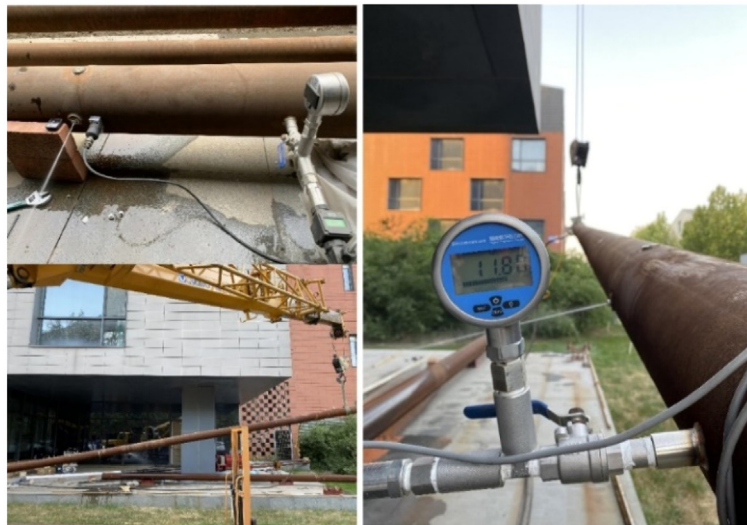
Fig. 2. Experiment apparatus and process: (a) The spherical detector (SD) used in the experiments and the leak plug dimensions; the SD is still and right below the leak point. (b) the SD is rolling down and passing by the leak point. (c) Experiment photos.
