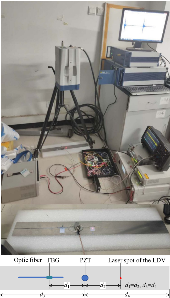
Figure 5. A schematic of the comparison experiment between FBG and the LDV.
